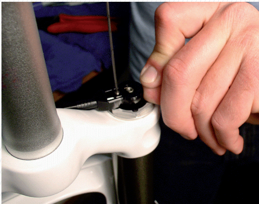
Figure 25: Tightening the Shimano Inner Cable Set Screw
