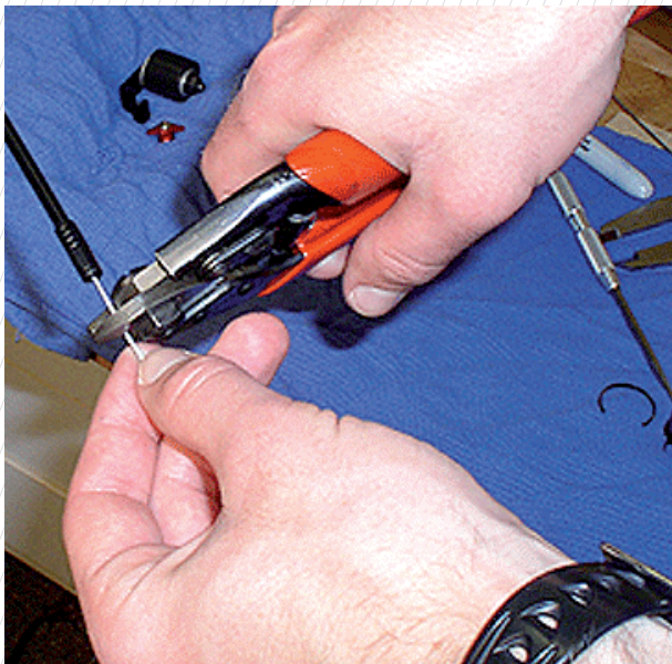
Figure 22: Cut the Exposed Inner Cable End to Specification
