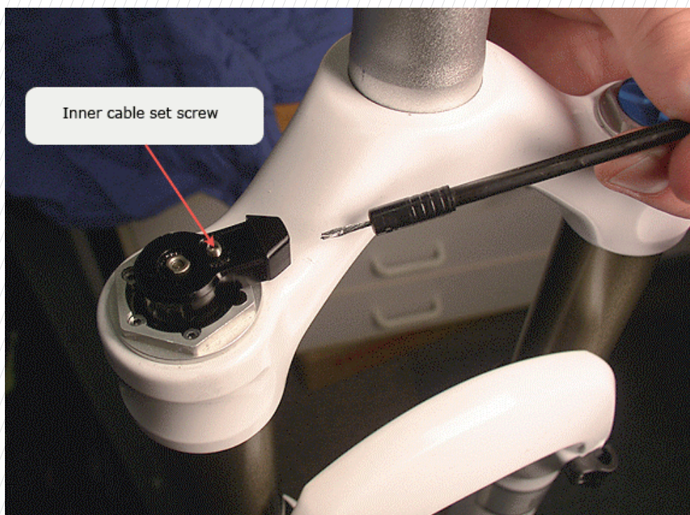
Figure 6: Remove the Inner Cable Set Screw
