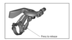
Change the modes by pushing the lever with your fingers frontward and release them by tapping the release button (one mode per push/release)
