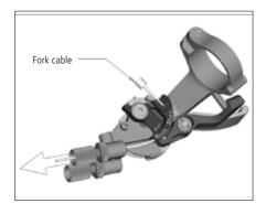
Fix the cable with the 2mm allen screw on the barrel adjuster on the fork crown with a tightening torque of 0.9Nm/ 8lb/in, cut the cable and secure it with a cable end-cap. Please refer for this action also to the manual of SRAM/RockShox attached to the bike.
