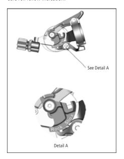
To assemble the cable please bring the lever into the All Travel Mode, push the cable into the lever-eyelet as shown on drawing below, push it through the pre-cut cable housing and fix it at the assembly unit on top of the right side of the fork crown.
