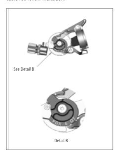
To assemble the cable please bring the lever into the Full (Travel) Mode
