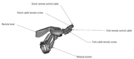
Regarding the installation and adjustment of the rear shock remote cable please follow the instructions of the different shox attached to your bike. Please note that the cable for the rear shock is ALWAYS the upper cable on the lever as shown in drawing below. There are 3 different versions for different rear shock models.
