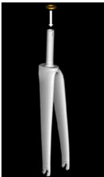
1. Assembly lower bearing on fork carbon crown
