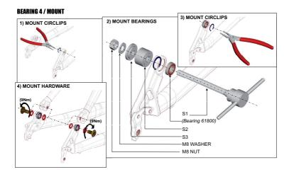
The bearings are standard size and can also be ordered in local hardware stores, in case customers do not want to replace all parts.
