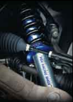
FORD F-150 SVT RAPTOR WITH FOX'S PATENTED INTERNAL BY-PASS TECHNOLOGY First production internal by-pass on an OE truck
