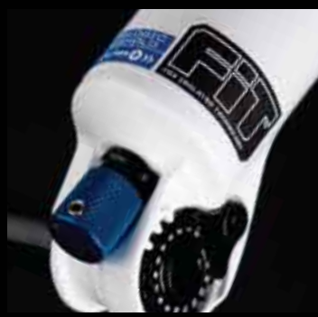
Terralogic threshold adjust located on bottom
