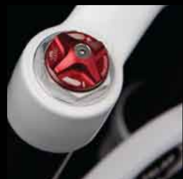
Rebound adjust located on top
