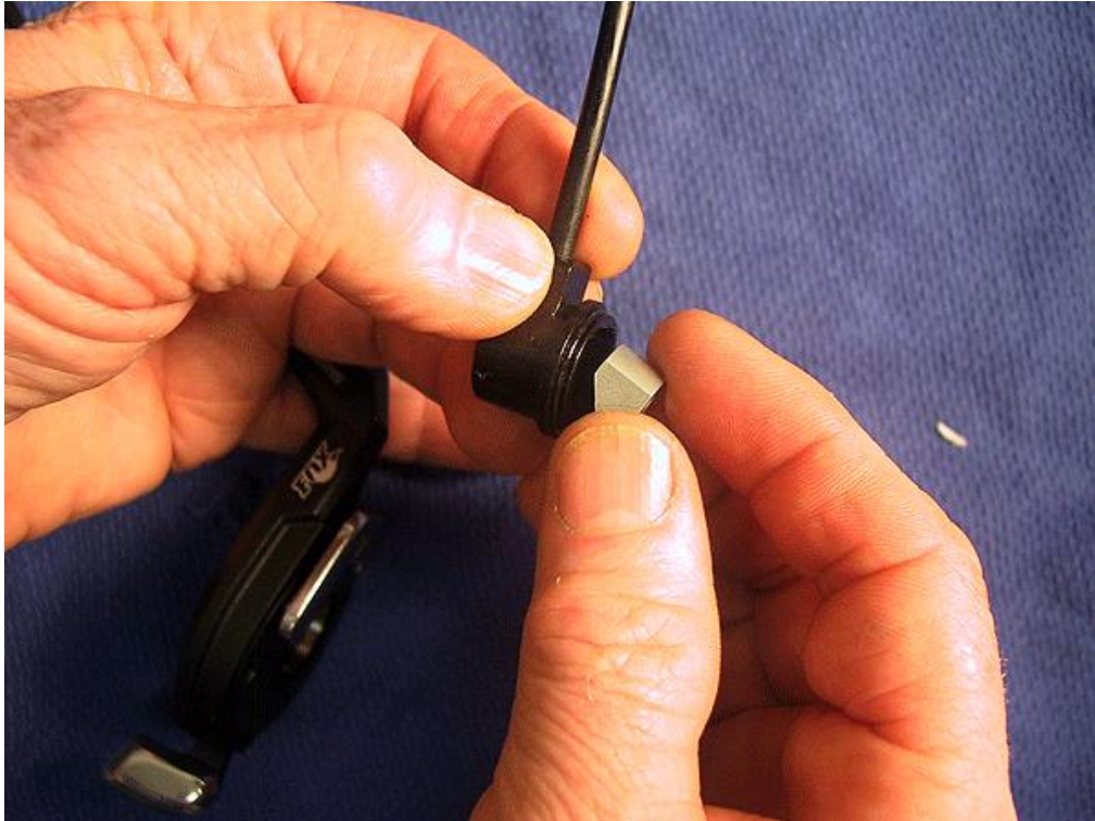
Figure 59: Removing the Lower Cam
