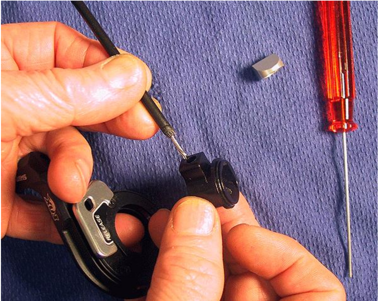
Figure 61: Removing the Original Control Cable
