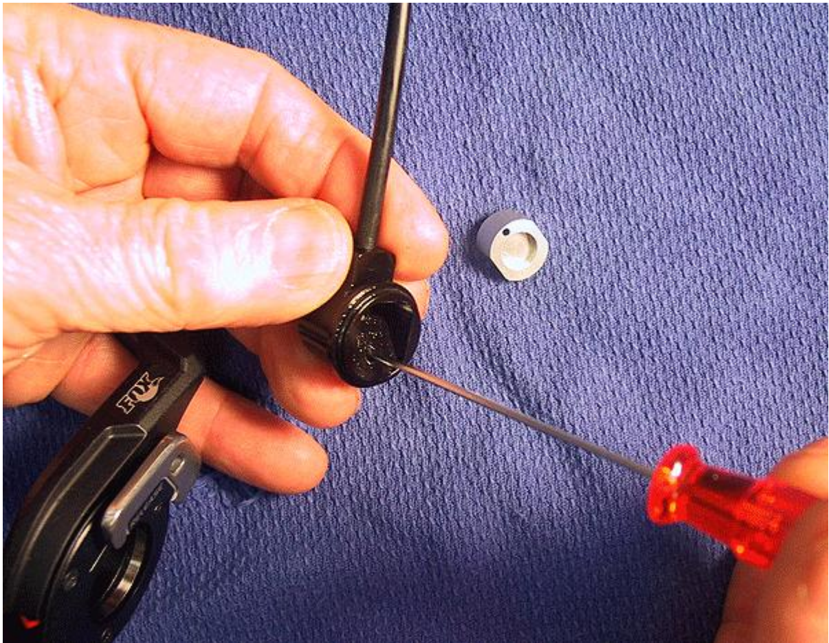
Figure 60: Removing the Inner Control Cable
