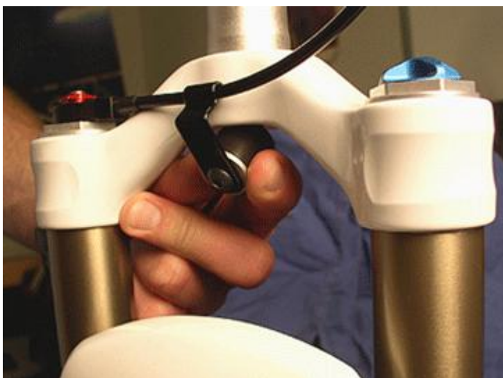
Figure 80: Cable Housing With Cable Holder Assembly
