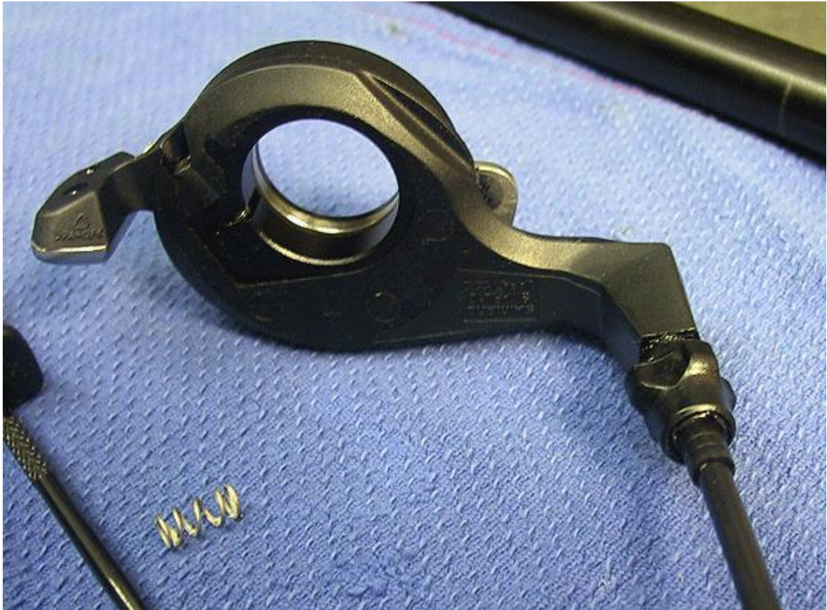
Figure 63: Remote Lockout Lever with Cable
