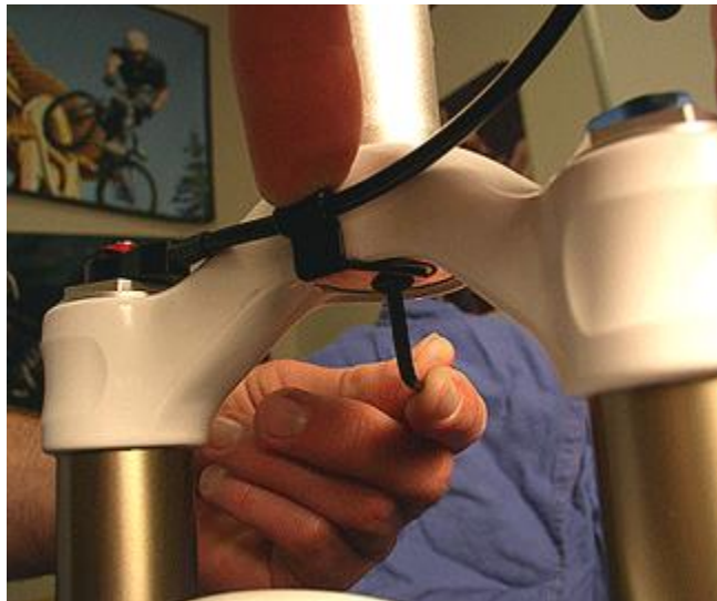
Figure 31: Securing the Cable Holder Assembly
