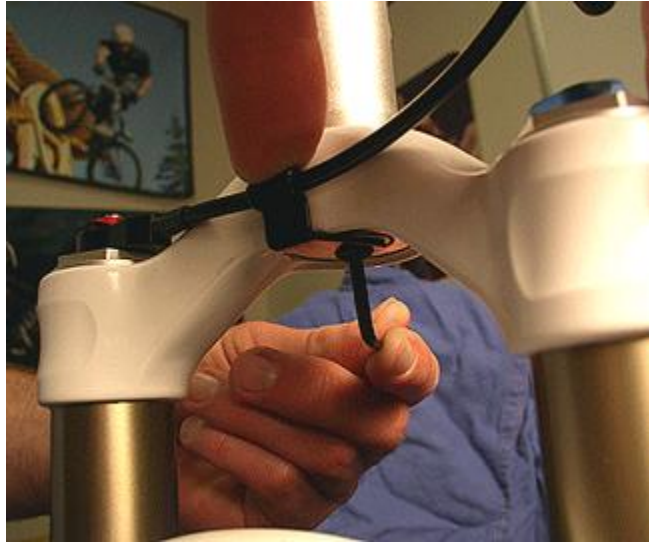
Figure 1: Removing the Cable Holder Assembly
