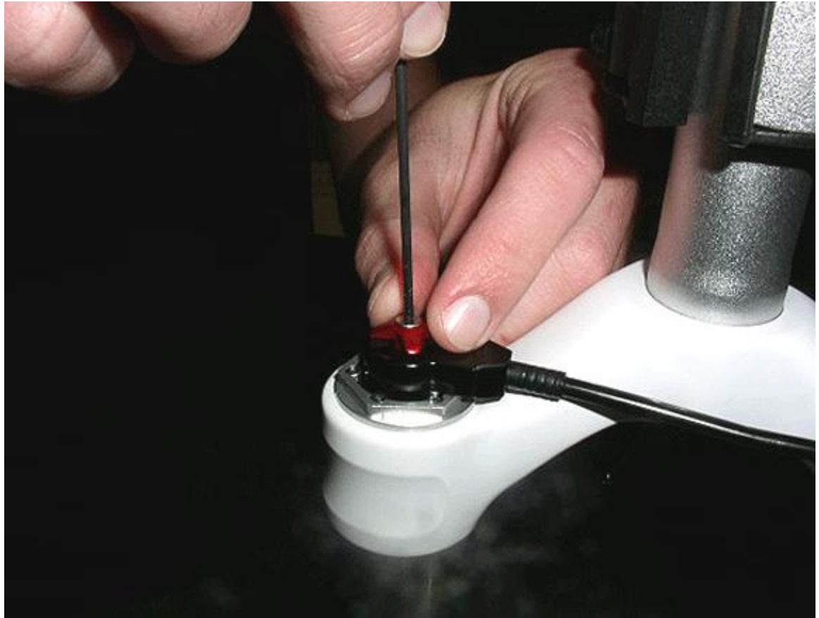
Figure 29: Installing the Rebound Knob
