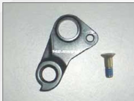
219577 Dropout Hang.right side IDS 2 142/RWS12
