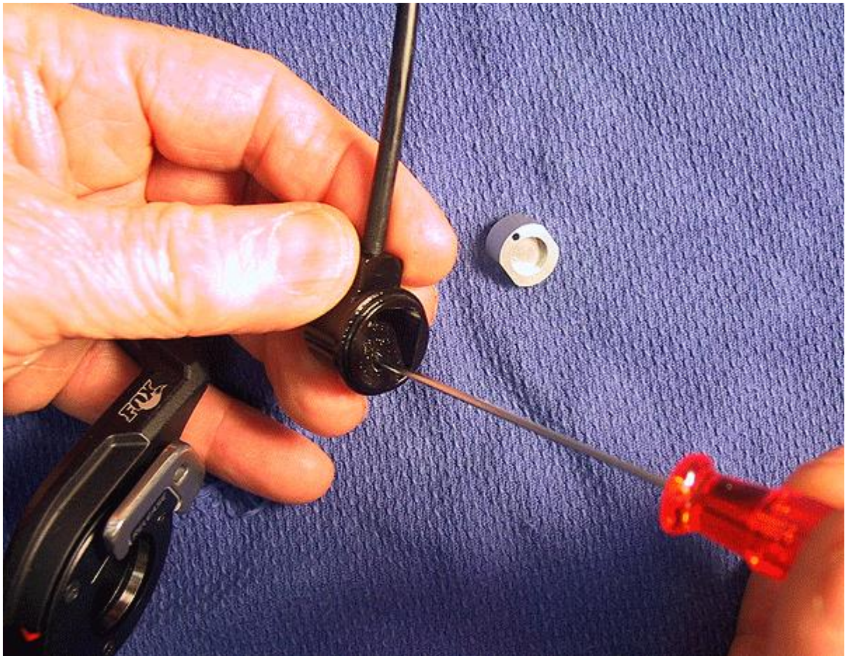
Figure 60: Removing the Inner Control Cable
