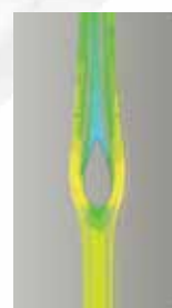
Late flow separation = limited drag
