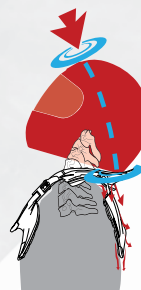
COUPLED AXIAL LOADING: Helps prevent axial loading only when the axial forces act in combination with other mechanisms.
