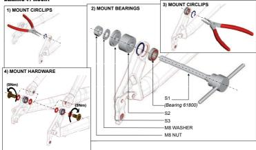
The bearings are standard size and can also be ordered in local hardware stores, in case customers do not want to replace all parts.
