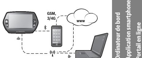
The diagram illustrates the communication network. The Nyon computer is connected via a GSM/3G module to both a smartphone and the internet (WWW). The smartphone is also connected to the Nyon computer via Bluetooth.
