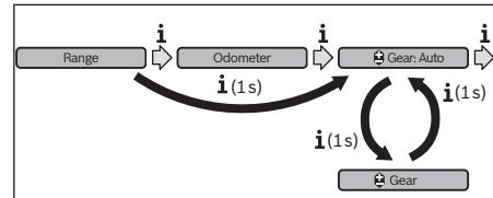
By pressing the “**i**” button for more than 1 s, you can switch back and forth between the “**Gear: Auto**” automatic mode and the “**Gear**” manual mode.
