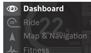
Press left on the joystick **1** to overlay the active operating mode with the main menu and to switch it to the main menu (see picture above).
