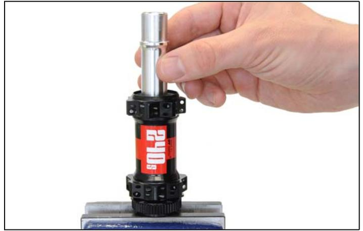
4. Put the dismantling tool onto the axle.
