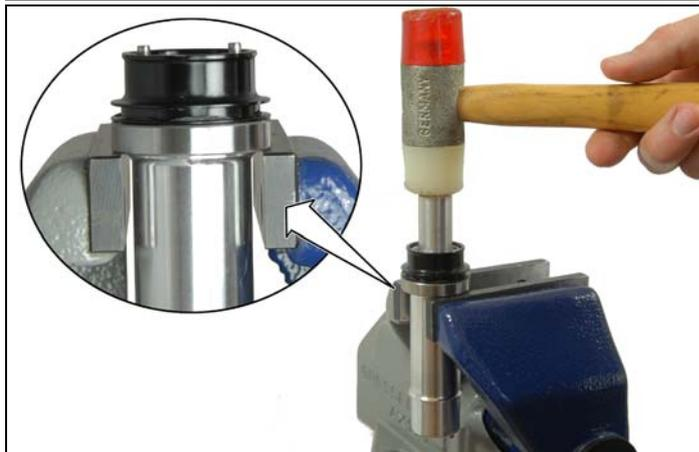
7. Put the axle into the second bearing.
