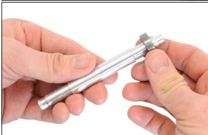
3. Slide the axle ([fig.4-4/3](#)) through the second bearing ([fig.4-4/2](#)).
