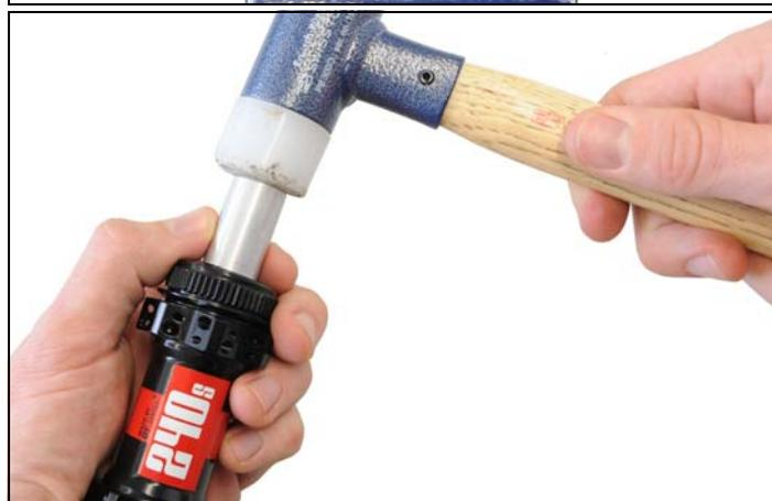
3. Put the axle into the hub shell.
