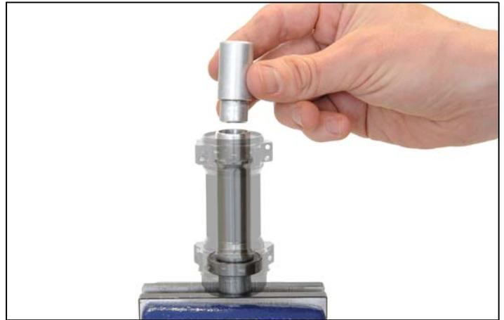
5. Tap out the second bearing (fig. 4-1/2) using the disassembly tool and a hammer.
