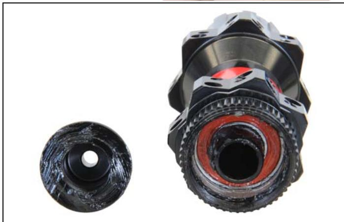
4. Put both adapters (fig. 4-6/1/13) onto the hub.
