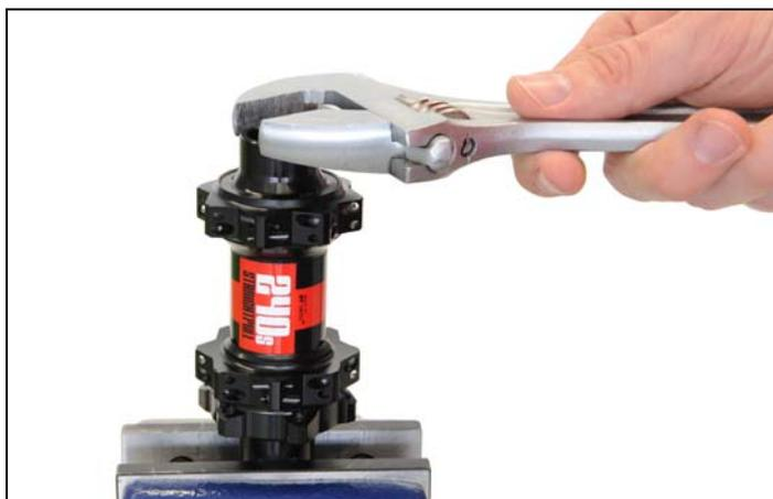
2. Slide the disassembly tool onto the axle ([fig. 4-3/3](#)).
