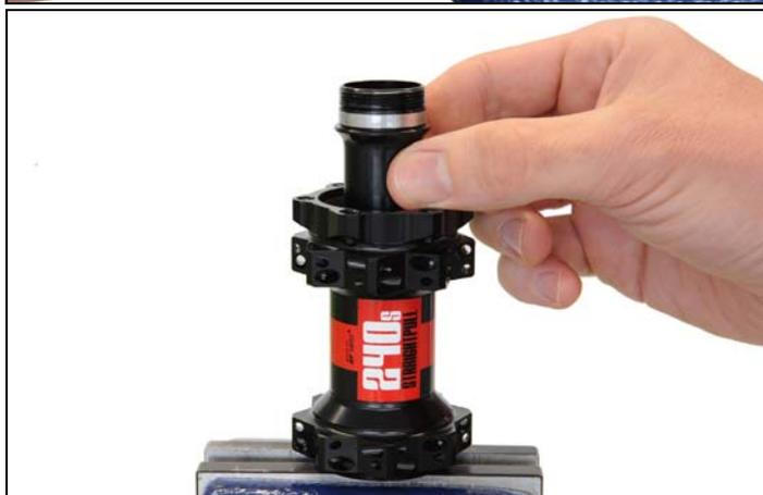
8. Tap out the second bearing (fig. 4-3/2) using the disassembly tool and a hammer.
