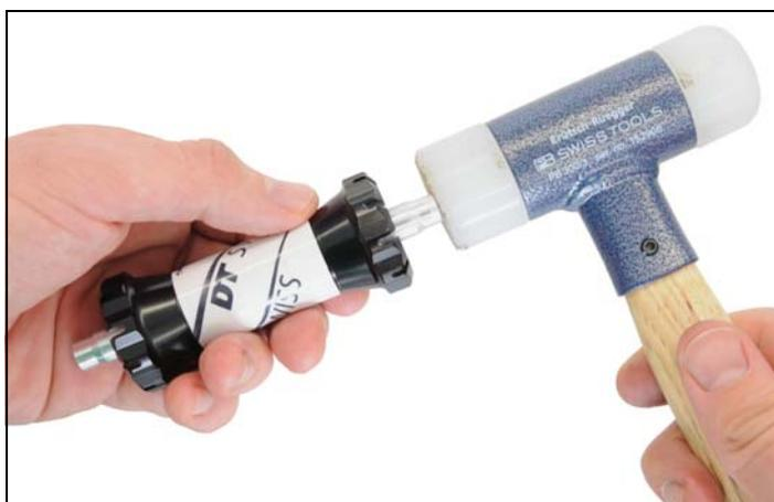
2. Pull the bearing ([fig.4-4/2](#)) off the axle ([fig.4-4/3](#)).
