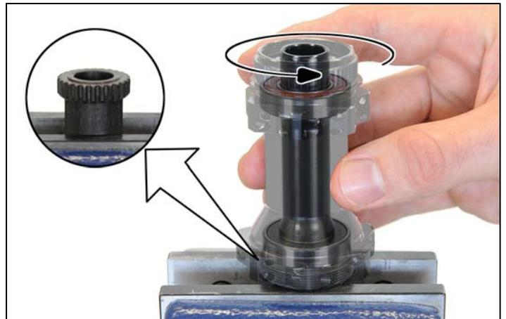
5. Remove the ring nut ([fig. 4-6/7](#)), the sealing ([fig. 4-6/8](#)) and the shim ring ([fig. 4-6/6](#)).
