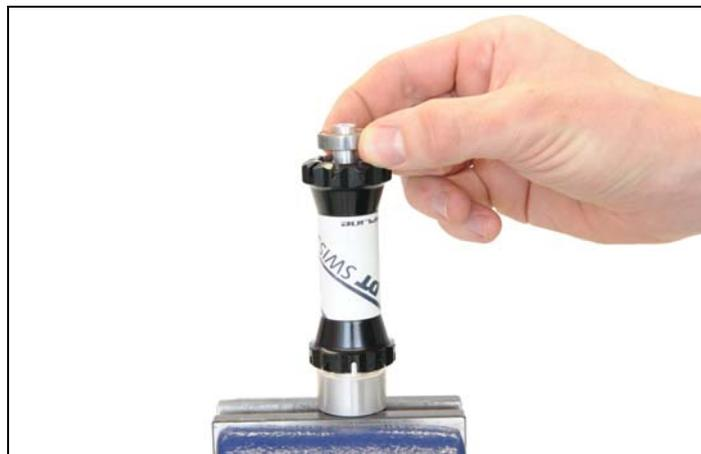
5. Put the second installation tool onto the bearing (fig.4-4/2) and tap in the bearing using a plastic hammer.
