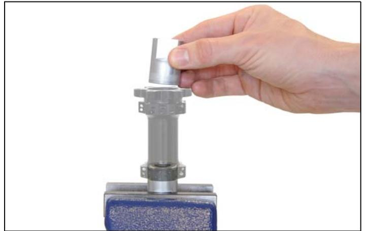
6. Tap in the bearing using a plastic hammer.
