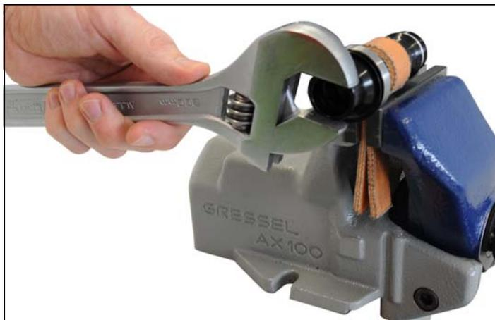
6. Remove the bearing from the axle.
