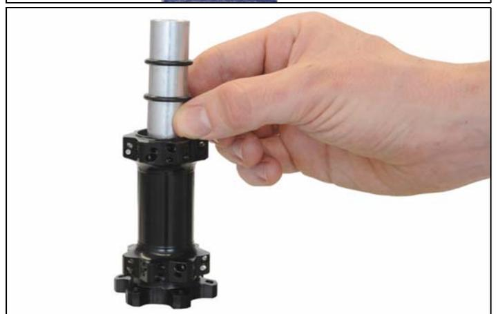
9. Put a new bearing (fig.4-5/3) with the colored side facing outwards onto the bearing seat.
