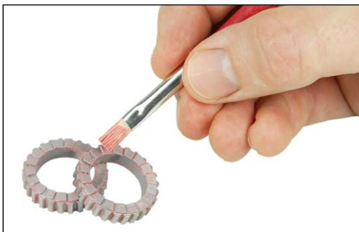
2. Grease the tooting of the rotor using DT Swiss special grease.
