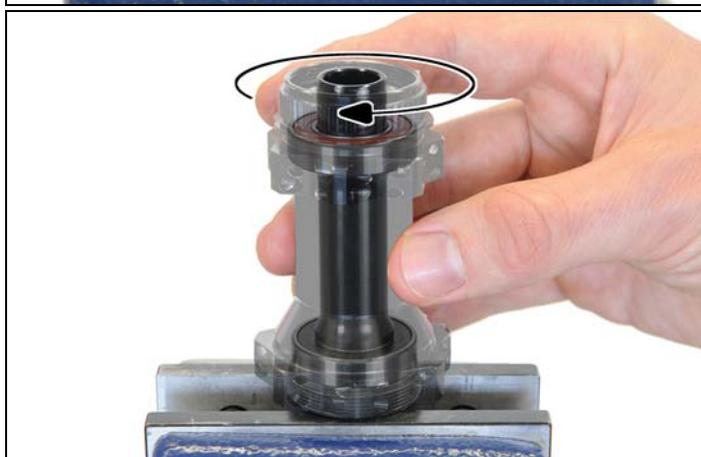
5. Release the ring nut tool, turn it 90° and clamp it into the vice in its high position.
