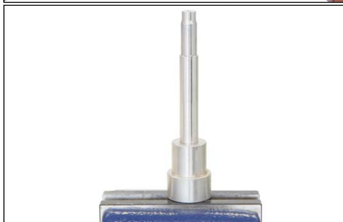
3. Slide the hub shell (fig.4-4/4) onto the installation tool and the axle (fig.4-4/3).
