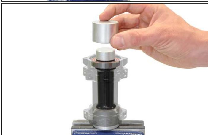
**7.** Tap the bearing into the hub shell with slight hammer strokes.
