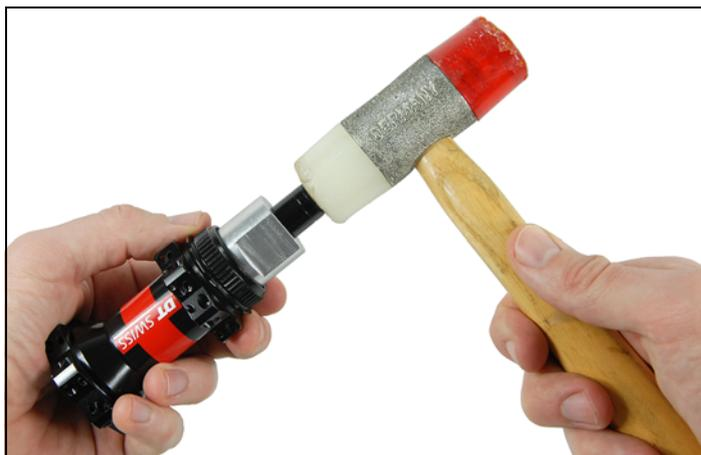
5. Remove the bearing from the axle.
