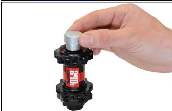
3. Tap the bearing ([fig. 4-3/2](#)) and the axle out of the hub shell using the disassembly tool and a hammer.
