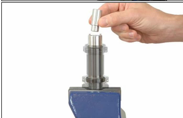
9. Tap out the bearing with slight hammer strokes.
