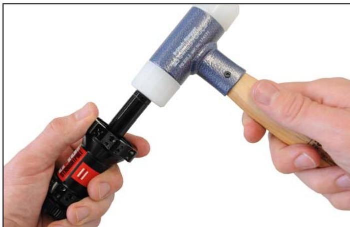
2. Remove the bearing from the axle.
