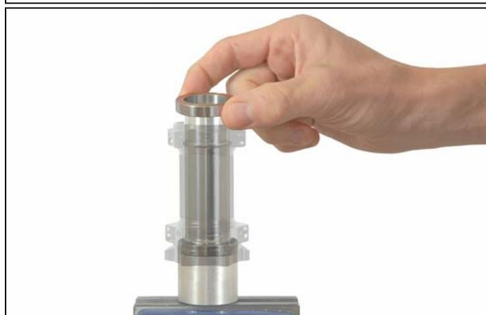
9. Put the second mounting tool onto the bearing on the non brake side.
