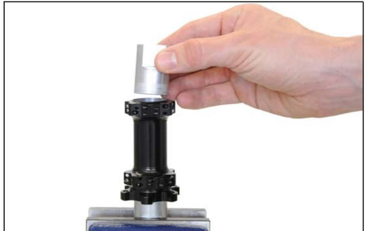
13. Tap in the bearing (fig.4-5/3) using a plastic hammer.
