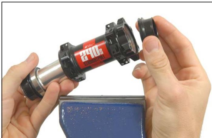
4. Open the clamping jaws of the vice that much that the bearing rests on the jaws, but the axle is not clamped.
