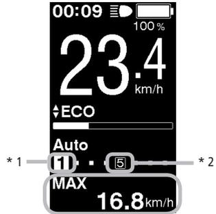
\*1 Gear position (displayed only when using electronic gear shifting)
