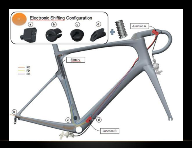
Install all Shimano components according to Shimano installation guidelines !!!!!!
