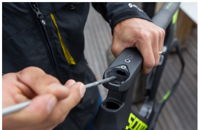
2 Again he removes sharp edges on the routing holes using his soft wire brush.
