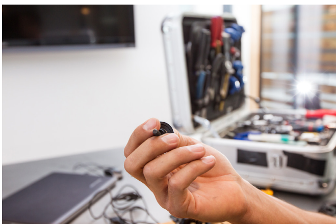
7 Apply a thin layer of medium strength Loctite to the screw of the inner compression cap. Note: do not use just any kind of grease, otherwise the headset could get loose.
