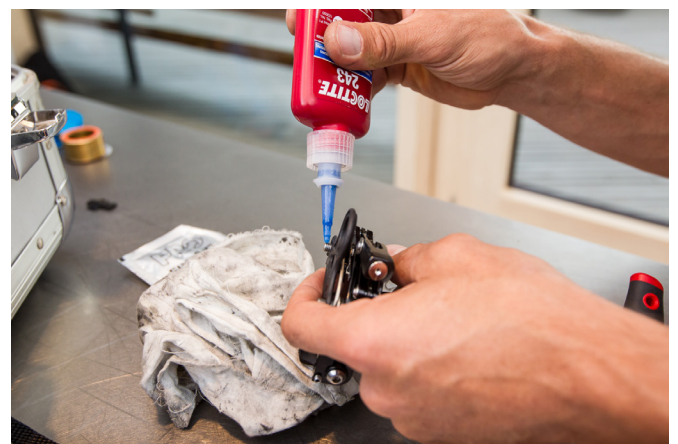
8 Apply a medium-strength Loctite to the pulley bolts.
