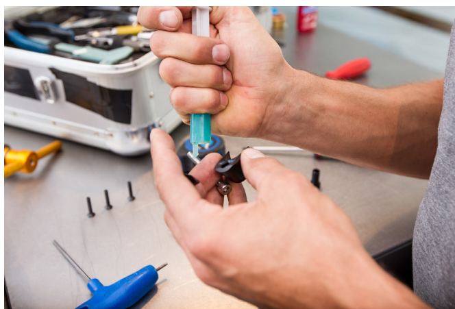
19 Treat clamping parts of metal with standard grease. Carbon surfaces in the seattube and on the seatpost require Dynamic's red fitting grease for carbon.
