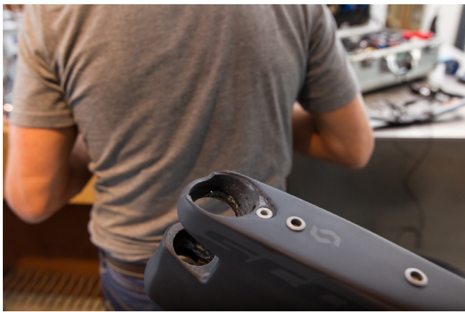
3 Before fitting the bearings, lightly grease the bearing carrier.
