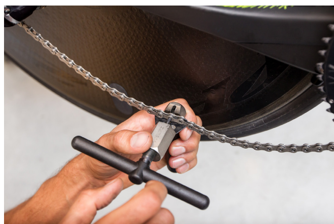
14 The chain has to be closed with a special joining link or a chain-riveting tool.
