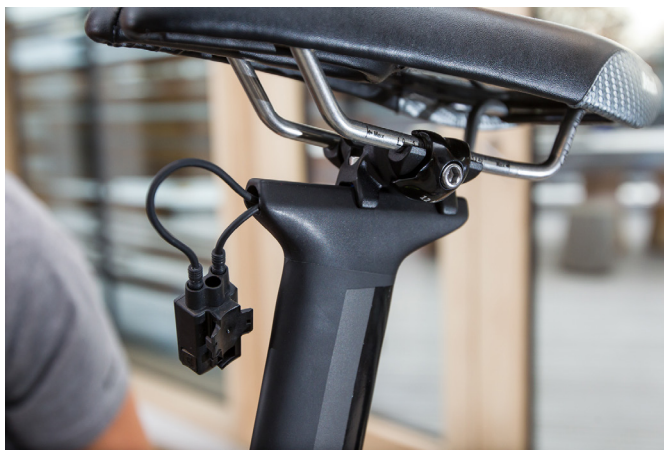
17 Attach the Di2 junction box below the saddle. This can either be done directly on the seatpost (with Loctite) or on the saddle rails (with cable ties).
