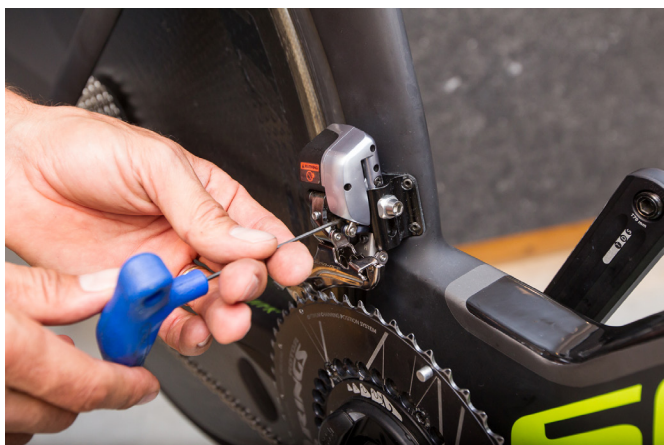
17 Set the height of the front derailleur so that there is a clearance of 1 - 3 mm between the chain guide outer plate and the largest chainring. Use a 5 mm Allen key to secure the chain guide's outer plate so that the flat part of the plate is directly above the largest chainring and the chain guide's rear edge is within 0.5 - 1.0 mm from the front edge of the chain guide. Use a 2 mm Allen key to turn the support bolt in order to adjust the position of the front derailleur, so that the flat part of the chain guide outer plate is parallel to the largest chainring. Adjust the inner and outer end stops of the front derailleur.
