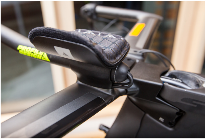
15 A rubber grommet protects the cables and keeps them in position.
