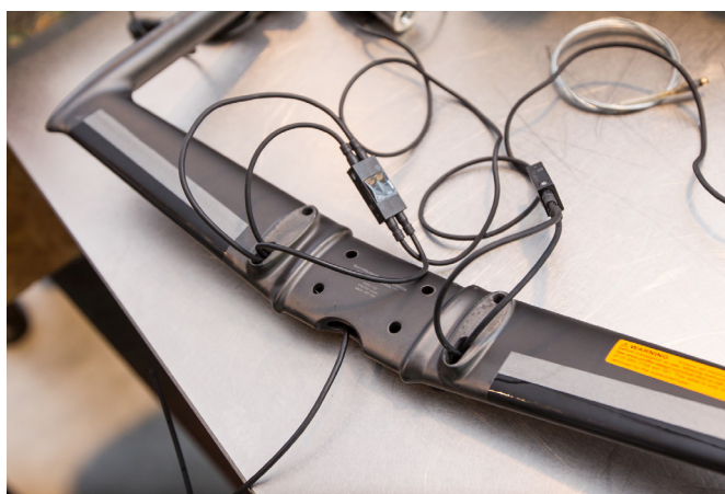
14 It doesn't really matter in which order you install the wires and cables, but it would be smarter to begin with the thin and flexible electric wires, followed by the considerably thicker brake cables.
