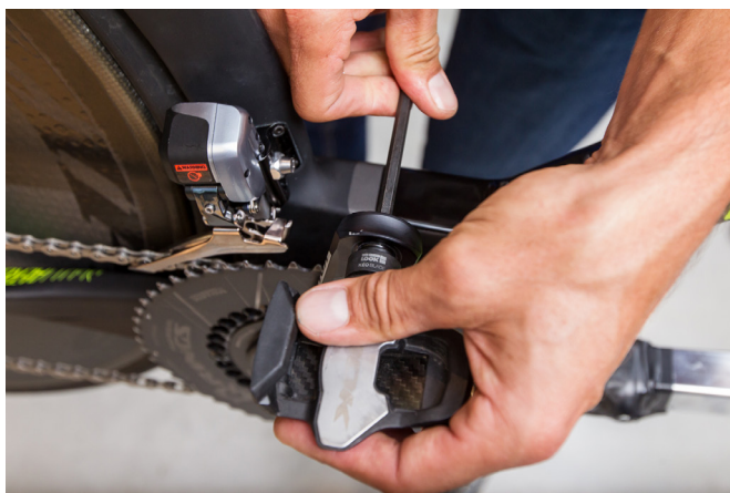
16 Mounted pedals simplify the rotation of the crank arms while adjusting the gears.
