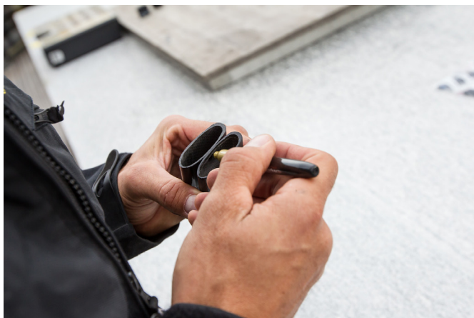
3 We mark both positions of the new mounting holes which are required for the flexible battery bracket...
