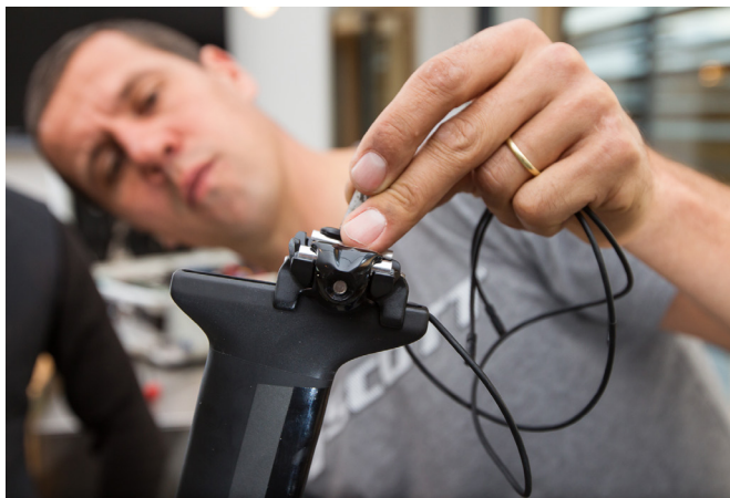
6 The wires of the junction box and the battery pack are routed from the top through the seat post.
