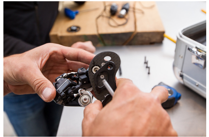
6 In an intermediate step we pimp the Shimano Di2 rear derailleur with the Berner Ceramic Cage.
