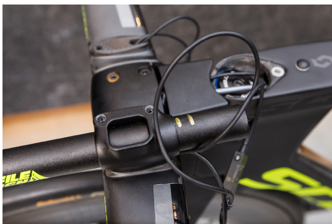
11 ... and cut them on the front or rear. Note: Do not notch the Di2 openings on the underside of the extensions.
