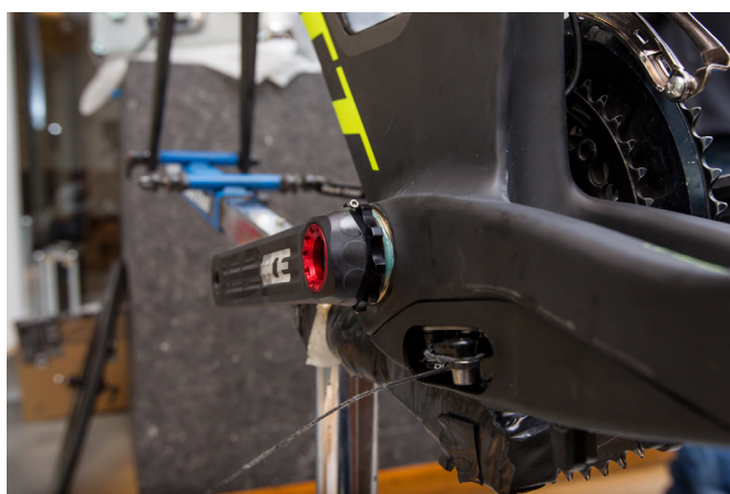
8 Adjust the preload on the non-drive side for smooth running and free clearance.
