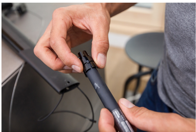
7 Put the battery pack into Scott's special battery bracket...
