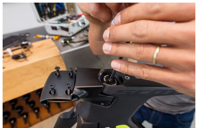
8 To adjust the headset, turn the top cap bolt clockwise until any free play is gone and the fork still turns freely.
