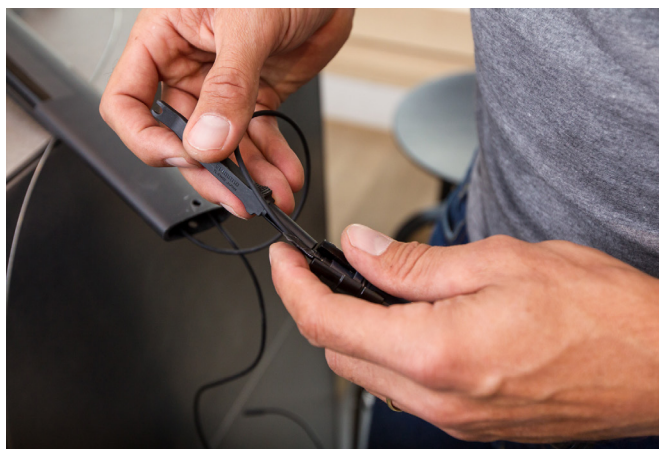
8 ... and connect the battery with the correct wire. Note: Make sure of clean and proper plug connections!
