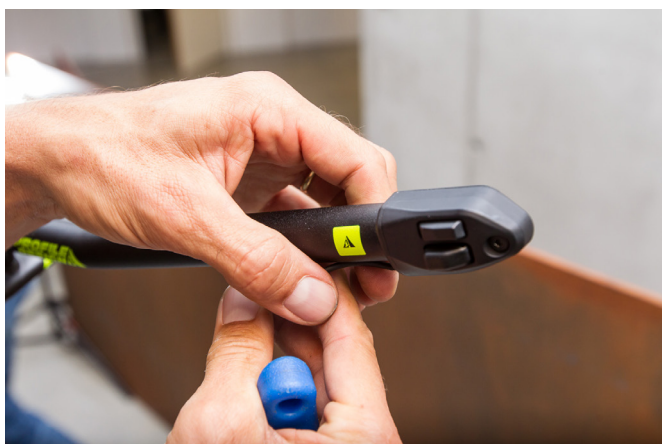
13 Install the shifters in the extension and adjust them to the desired angle.
