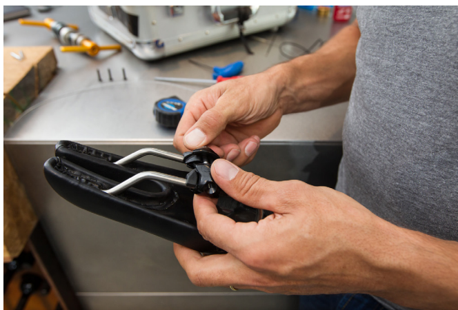
15 The clamp works with round and oval saddle rails.
