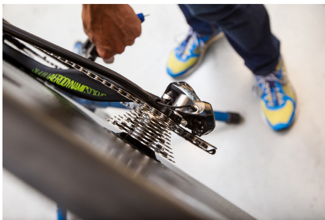
18 Finally, adjust the inner and outer end stops of the rear derailleur and fine-tune the Di2 gearing system in accordance with common practice and Shimano's instructions.
