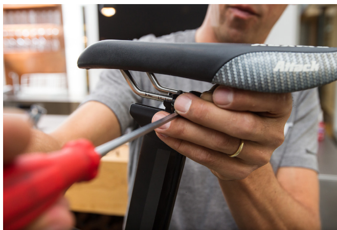
16 Adjust the seat slider as well as the saddle position and tighten the Allen bolt with a maximum torque of 12 Nm.
