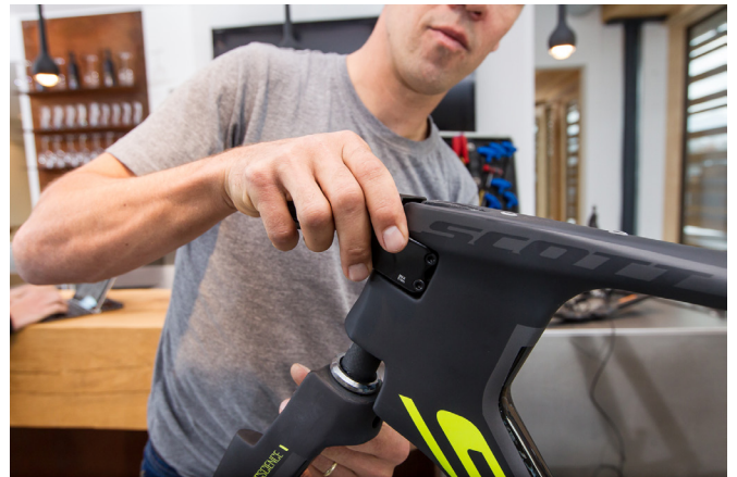
6 As Lars installs the fork from below the head tube, he slides the TT stem onto the steer-tube at the same time. The inner surface of the clamping area has been treated with the red Dynamic fitting grease for carbon.
