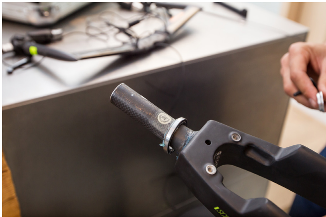
5 Slide the lower bearing directly onto the fork carbon crown. There is no additional crown race needed, but grease in between is a must.
