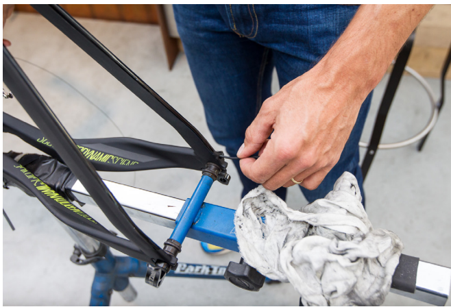
3 Route the rear derailleur wire through the dropout and chainstay...
