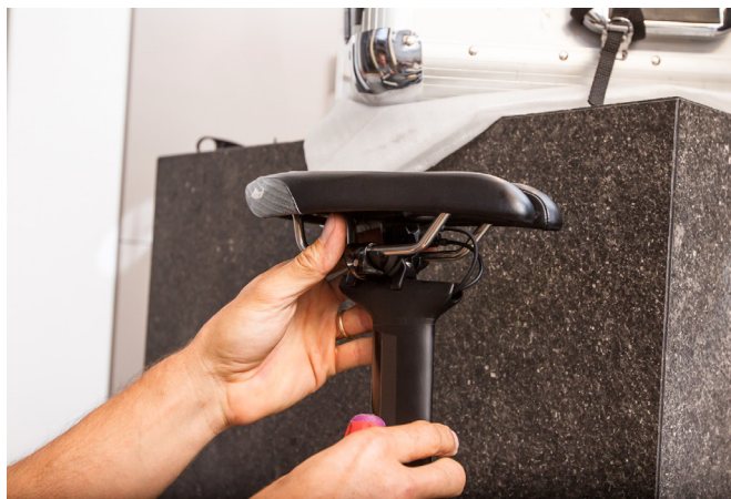
18 Our ISM saddle offers sufficient space to attach the junction directly on its rails.
