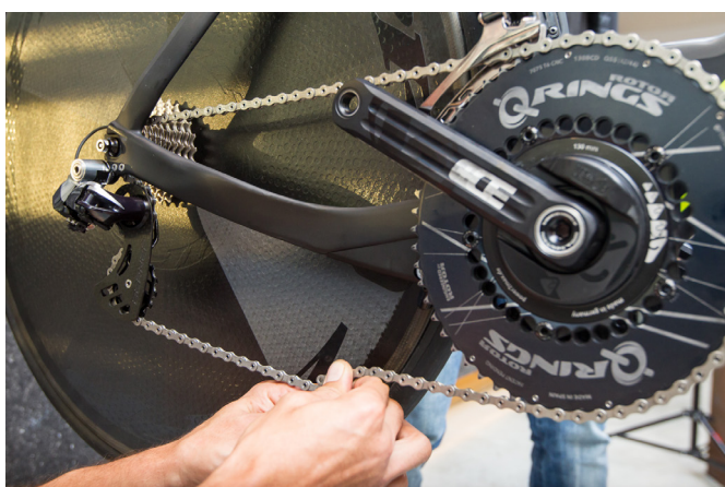
13 Determine the optimal length of the chain. (Note: the longer the better)
