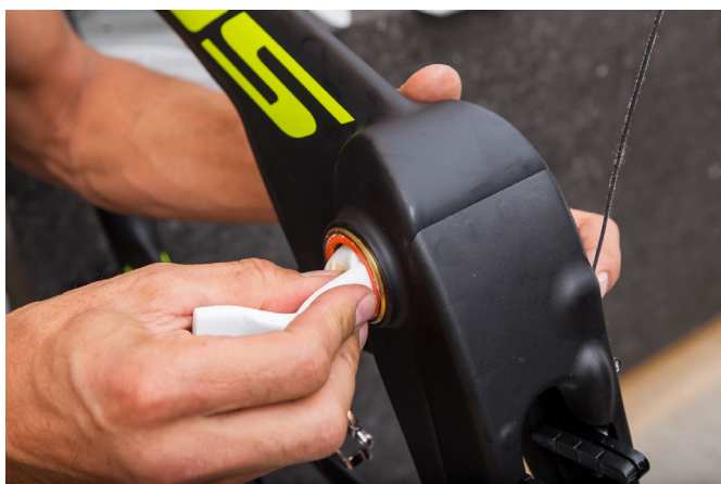
5 Recommendation for our special Rotor 4130 bottom bracket solution: to avoid rattling and chafing of wires against the axle, Lars inserts a small piece of foam into the down tube. In case of Shimano's and SRAM's press-fit bottom brackets this is not necessary, because they feature a one-piece protective sleeve.
