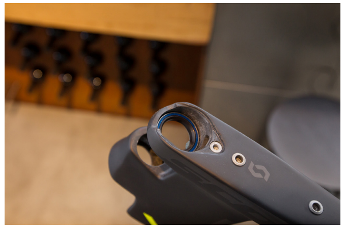
4 First the upper bearing is inserted into the head tube.
