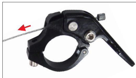
2. Pull until the end of the cable stops inside the lever.
