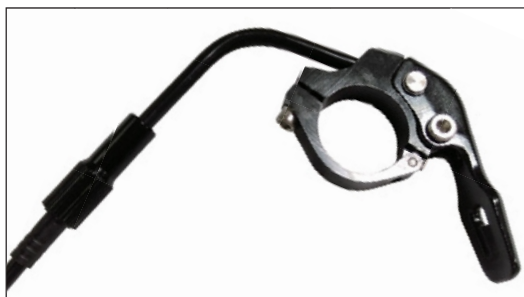
5. Pull through the cable until the rotary ferrules connect to the clamp lever.
