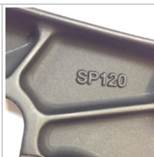
The linkage can be identified from markings on the inside 100/120
