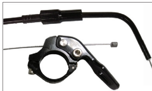
4. Insert the cable into the cable housing.
