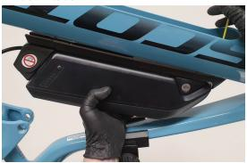
**25.**Ensure mounting bolts/ washers are fitted as shown
