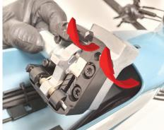
15. Remove x4 motor cover screws.
