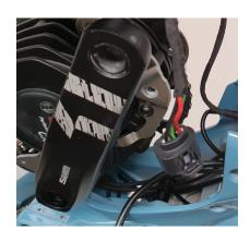
**32.** Connect both battey cables to Bosch Y cable 0275.007.930. This is the cable from the boost and original battery.
