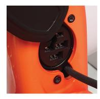
**E:** Cut the rubber charging cover to suit where the slot in the frame is.
