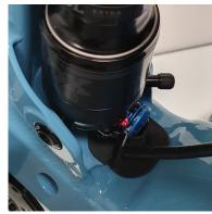
**30.** Unplug the battery cable from the rear of the engine
