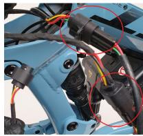
**33.** Pass the remaining Y connnector back between the motor and frame. **!DON'T CONNECT TO THE MOTOR!**
