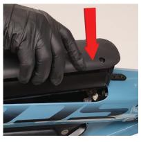
**39.** Fit "No Charge" decal over the additional charge port on the boost battery
