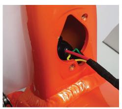
D: Refit the charging plug 4NM
