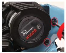
**18.** Slacken the rear motor bolt (do not remove).
