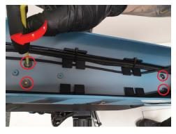
**27.** Route the cable from the battery through the shock hole.
