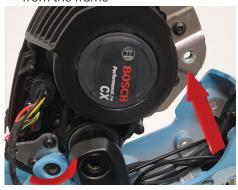
**20.** Rotate the front of the motor away from the frame
