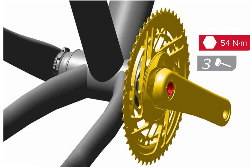
1. Apply grease to the spindle.
