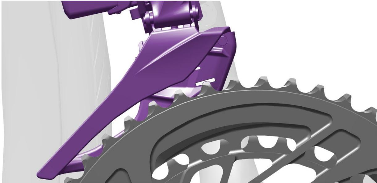
1. Adjust the derailleur so that the tip of the tallest chainring tooth appears within the setup line when viewed directly from the side.
