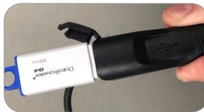
2. Connect the USB stick to a GCU (the GCU must be turned off, disconnected from the charger and the bike).
