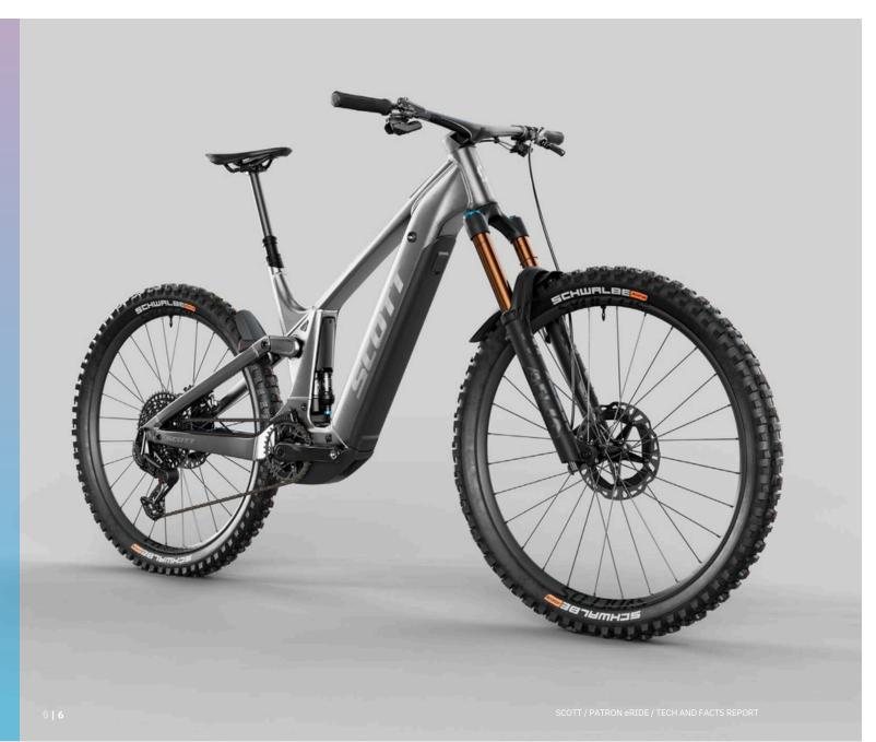
Balance is key and the Patron's geometry offers the perfect blend of Both the Patron and Patron ST feature 150mm of rear travel, with the 900 fun, control, efficiency, and comfort. It's designed to give you matching that in the front. The ST, however, is equipped with a 170mm confidence and agility on downhills while enabling powerful riding and fork, offering extra travel for added control and slackening the geometry efficient climbing with motor assistance.
